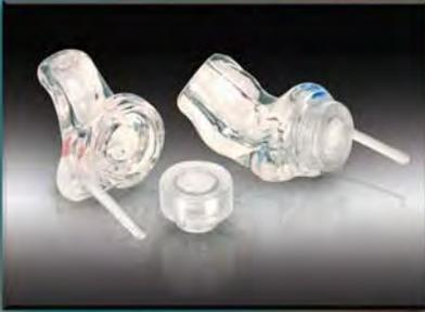
**Musician's Filtered Plugs** replicate the natural response of the open ear. Sound heard with these earplugs has the same quality as the original, only quieter. Accurate sound reduction is achieved by combining a patented filter with the specific acoustics of a custom earmold. Three attenuator filters are available: ER-9, ER-15 and ER-25. (The number corresponds with the amount of sound reduction in dB.)
